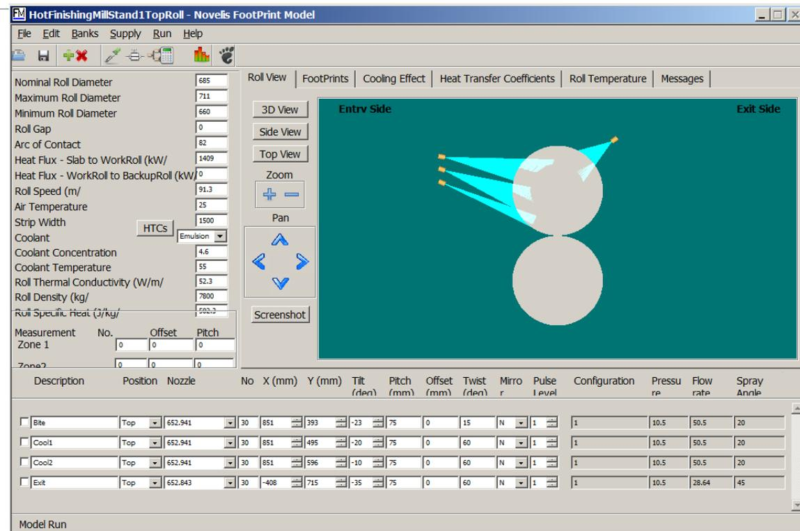
Interface for Footprint roll cooling design model
