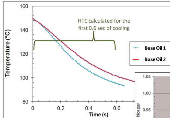
Cooling curves measured with two base oils
