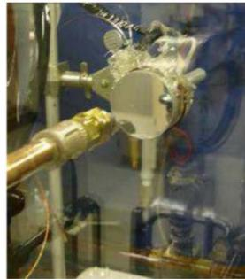
Lab rig for measuring cooling performance of lubricants
