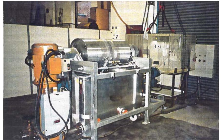
Rotating roll rig for roll cooling measurements
